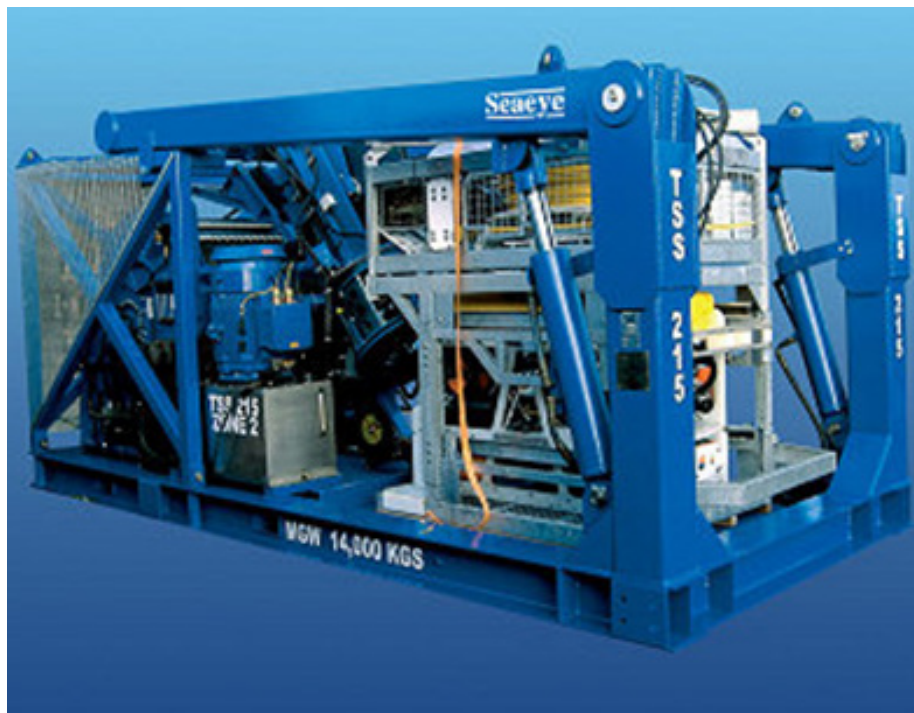
LARS in stowed position with TMS and Cougar ROV ready for transport
