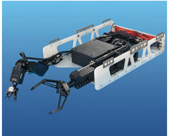
Five-function manipulator and three-function grabber skid
