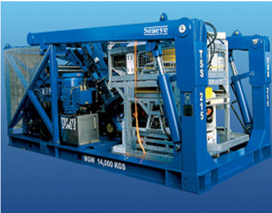
LARS in stowed position with TMS and Cougar ROV ready for transport Cougar TMS & LARS with Snubber Rotator
