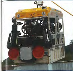
Global Diving & Salvage Inc's custom-developed skid, fitted with the neutron backscatter tool, was deployed to determine the presence of oil aboard a sunken vessel.
