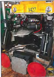
The neutron backscatter tool fitted on Global Diving & Salvage Inc's custom-developed skid.
