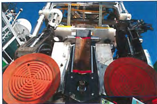
(Top) Global Diving & Salvage Inc.'s sampling tool system, with suction cups fitted to Saab Seaeeye's Cougar ROV.
